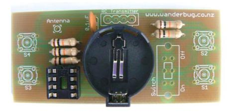
3. Fit and solder the main switch and the four push-button switches in place. Make sure all switches are pushed in fully before soldering.
