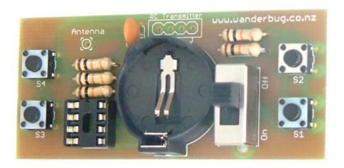
4. Snip off the excess pins on the **Dorji** transmitter module so that it will fit snuggly in beside the battery holder, and solder in place.
